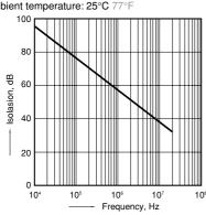
14. Insertion loss vs. frequency characteristics (50 $\Omega$  impedance)
